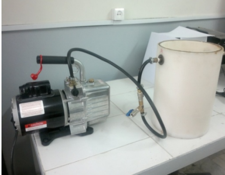
Figure 2 – Vacuum chamber and pump used in this study
