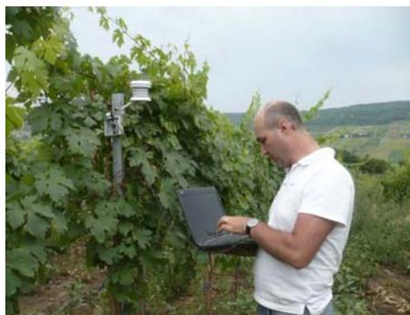
Figure 1 - Tinytag TK- 4014 temperature loggers in Cotnari vineyard
