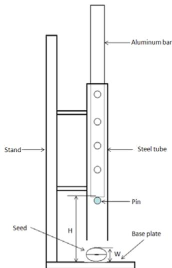
**Figure 1 - Schematic diagram of the impact test apparatus**
