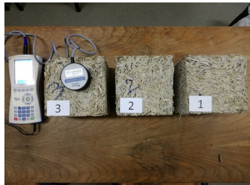
Figure 5 - Measurements of the heat transfer coefficient
